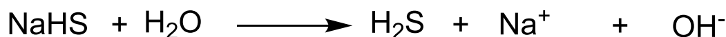
Fig. 2. Chemical structures and hydrolysis-based release mechanism of hydrogen sulfide (H 2 S) from disodium sulfide (Na 2 S) and sodium hydrogen sulfide (NaHS). Both salts liberate H 2 S upon dissolution in aqueous solution through simple hydrolysis.
